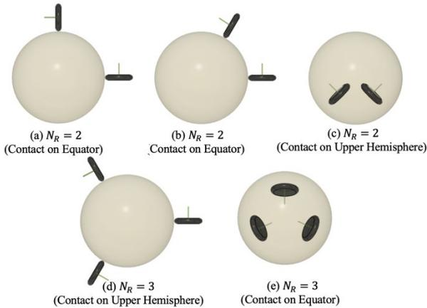
Figure 1. A pattern of roller arrangement for sphere mobile robot driven by multiple rollers.
