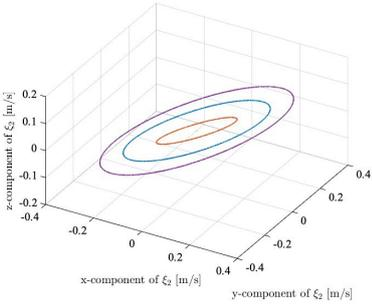
Figure 7 The trajectory of slip vector from sphere and roller  $\zeta_{2,k}(k = 1,2,3,4)$ .
