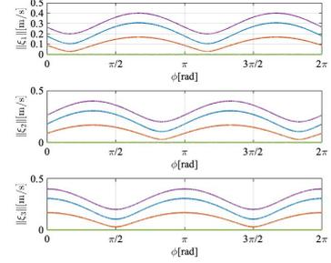
Figure 9 The slip speed of slip vector from sphere and roller  $\|\zeta_{1,k}\|, \|\zeta_{2,k}\|, \|\zeta_{3,k}\| (k = 1,2,3,4)$ .
