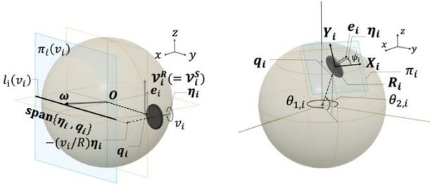
(a) The existence of sphere angler velocity vector in the case of a single-constraint roller. (b) Roller's axis vector  $\boldsymbol{\eta}_i$  at contact point  $\mathbf{q}_i$  on the sphere
