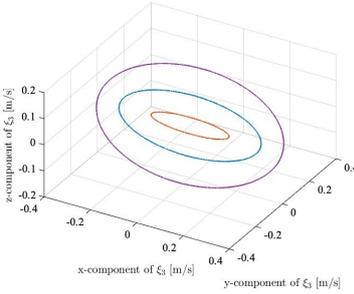
Figure 8 The trajectory of slip vector from sphere and roller  $\zeta_{3,k}(k = 1,2,3,4)$ .
