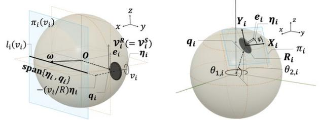
Figure 2 (a) The existence of sphere angler velocity vector in the case of a single-constraint roller. (b) Roller's axis vector  $\eta_i$  at contact point  $q_i$  on the sphere
