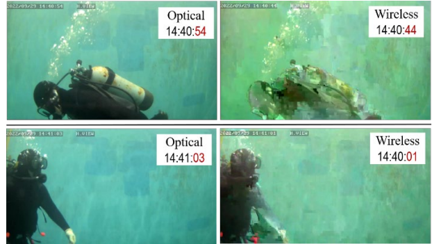
Fig. 9. Snapshots from the received videos when z=1m , (Mismatch timestamp when the same frames).
