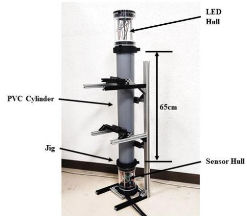
Figure 7: Experimentation Setup
