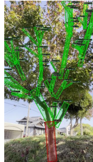
Figure 9 YOLO-OBB Prediction Results for Trunk and Branch Detection (Red boxes denote trunks, and green boxes denote branches)
