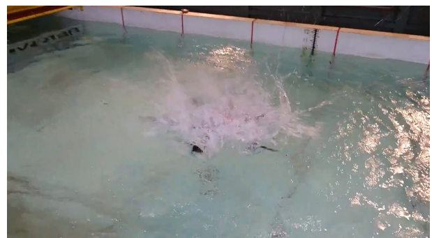
Fig.3 Diving of the UAV drone into the water
