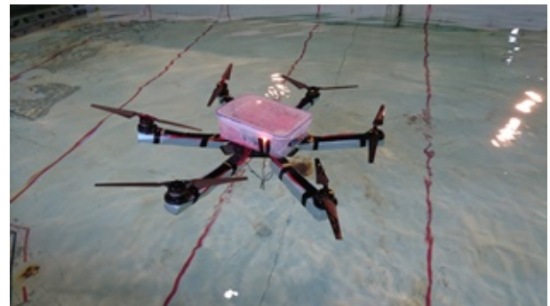
Fig.2 Electrical component in a watertight container
