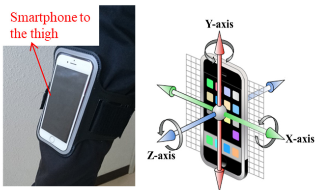
(a) Attached location (b) Smartphone axis information
