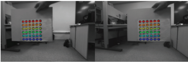
Figure 11 | Calibration of the robot's stereo pair with a circle grid in ROS (images are shown in grayscale)
