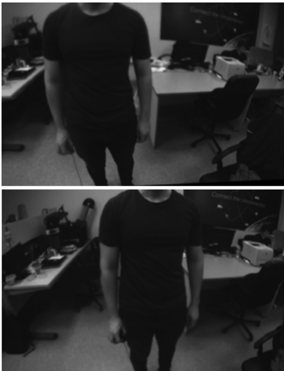
Figure 13 | Servosila Engineer's stereo pair calibration result (rectified and undistorted images). Part of loss pixels is truncated
