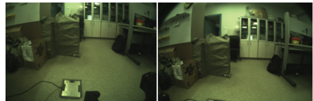
Figure 9 | Pictures taken from the left and right cameras of the robot's stereo pair (the center of the right camera is higher than the left camera)
