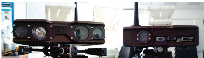
Figure 2 | Servosila Engineer's front and rear view cameras
