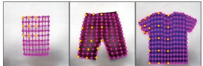
Figure 8 Sample of particle-based polygonal model is extracted for each category of garment. Selected particles defining the poses of the hanging garments. Orange markers define the poses on real garments from the particle-based model.
