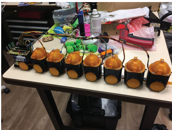
Figure 7 | Picture of the snake robot with the locomotive and the seven wagons.
