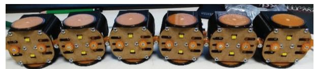
Figure 4 | The orange screw allows the tuning of distance of the different wagons but also the angle for the movement.
