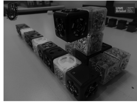
Figure 3 | Logic gates implemented with Cubelets.
