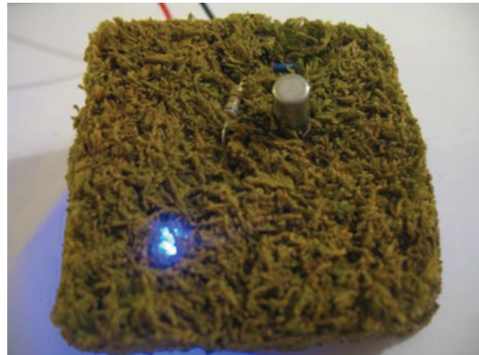
Figure 4 | A detail of a sense-and-actuate module to be mounted on PixelBeing' suit. Later prototype. A biomaterial-based circuit made out of natural wood and moss.
