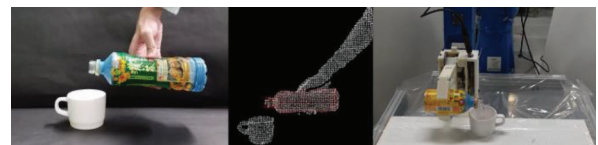
Figure 5 | Vision system for measuring object motion grasped by human and robot motion generation using the motion data.
