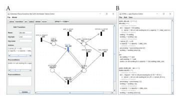
**Figure 5** | Screen shot of our prototype tool. (A) EPNAT model editor. (B) VDM++ specification editor.
