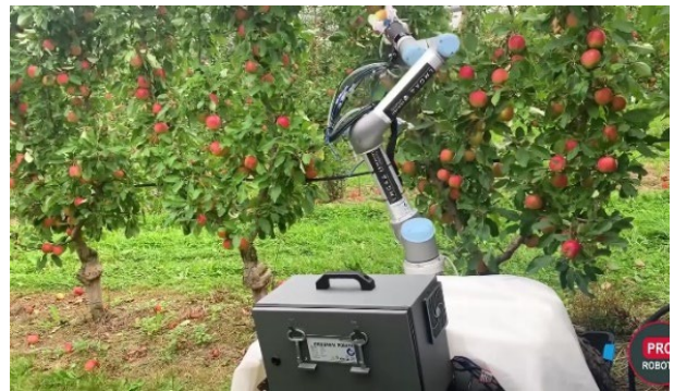
Figure 2. A new apple picking robot.
