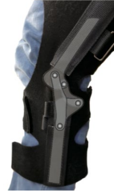
Fig. 2. A prototype exoskeleton-type knee joint support device [15].
