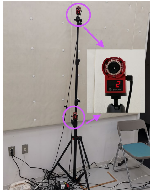
Fig. 2. Two OptiTrack Flex 3 cameras were installed on one camera stand at different height levels
