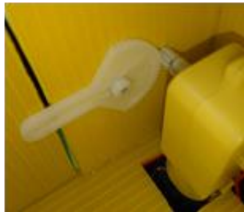
Figure 7: DC motor connected to the lock
