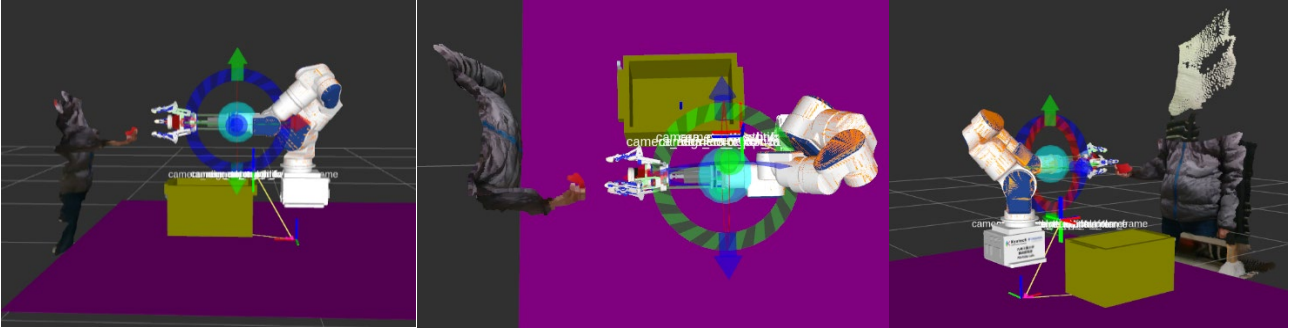
Fig. 5. 3D point cloud of environment and subject with robot model during handover experiment in different views
