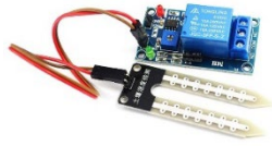
Fig.5. Soil moisture sensor
