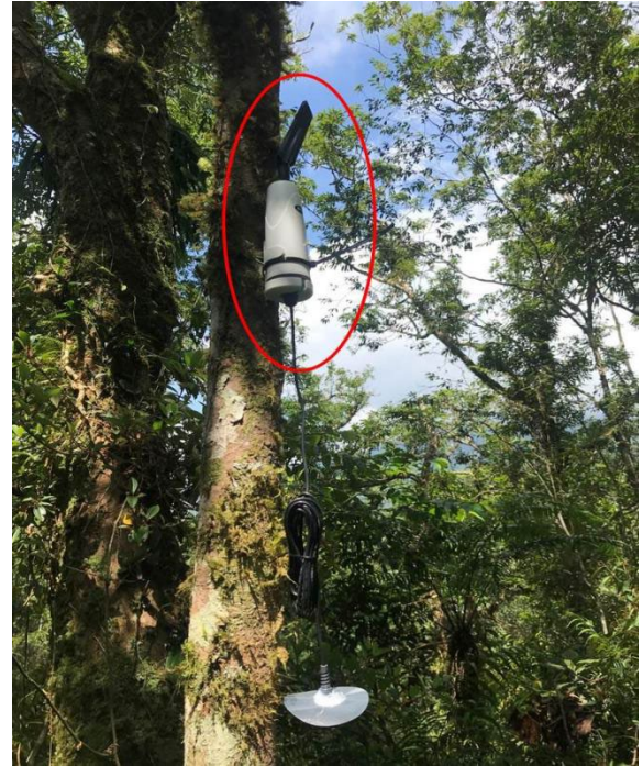
Fig. 5. NB-IoT-support temperature and humidity sensors.
