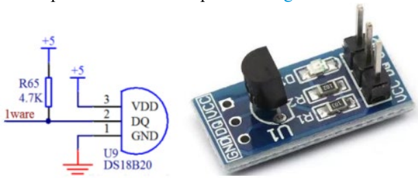
Fig.11 DS18B20 temperature sensor circuit schematic
